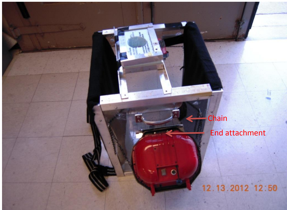
Illustration 4.9b. End attachment and using chain in LED installation.
